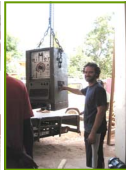
Using the new chain fall to unload the 800 pound welder.
