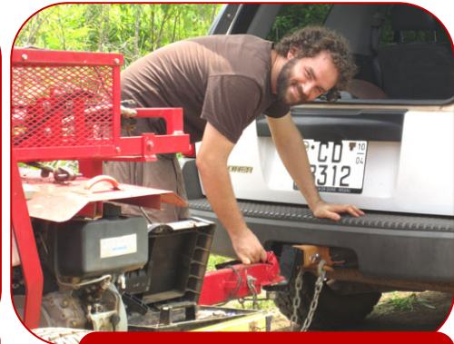
Getting ready to bring the block maker back from the village of Mansoa. You can see the bright orange hitch receiver Jason welded and installed. Eventually it will get painted black
