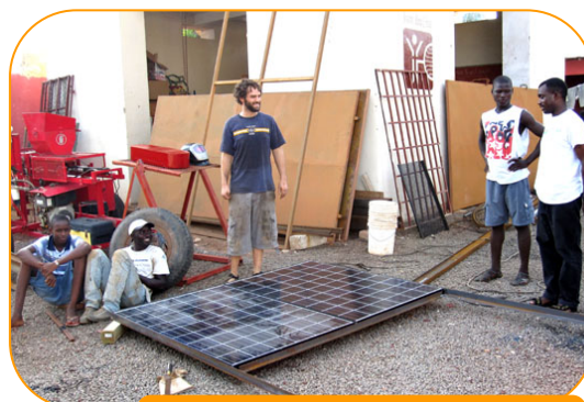
Testing the spacing on the prototype mount for the solar panels
