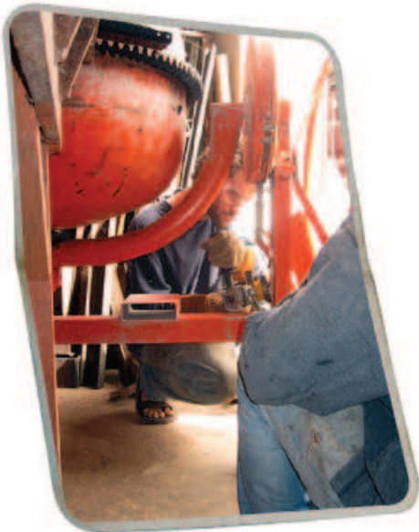
Reinforcing a broken cement mixer for a church construction project.
