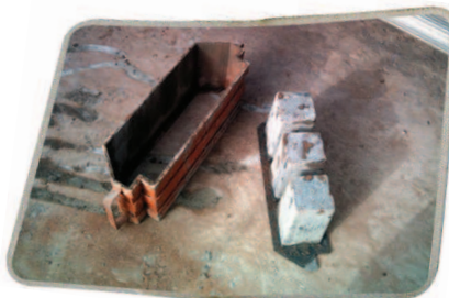
We made this form which is used to make a special kind of cement block by hand.
