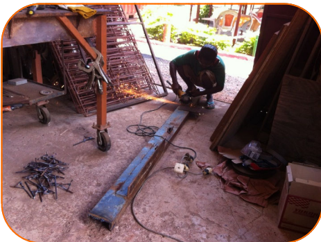
Grinding the steel they cut apart from the scrap yard into straight usable sections.
