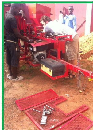
Repairing the compressed earth block making machine
