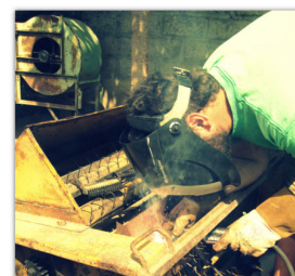
Using the welder to make some repairs on a hand-operated threshing machine.
