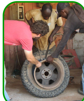
Jason was amazed that they were able to patch the gashed sidewall in our tire. In the US that tire would've been junk
