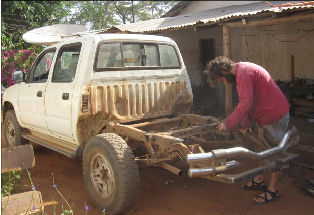
When the trailer hitch mounting bracket broke loose from the truck, they popped the box off and Jason welded it back on.
