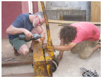
This pallet jack broke as we were unloading the container and we couldn't get spare parts here. So Bill had a custom hose made the next day and brought it with him and they got the pallet jack working again.
