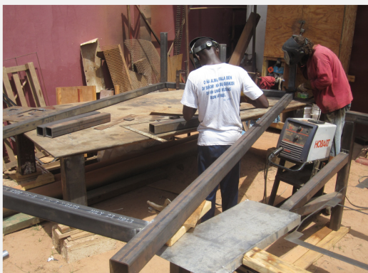
Jason's intern, Widafa, got a lot of welding practice making the plasma table.
