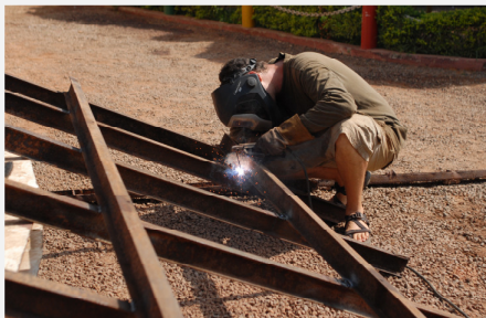
Jason welding some i-beams to support the deck on our trailer.
