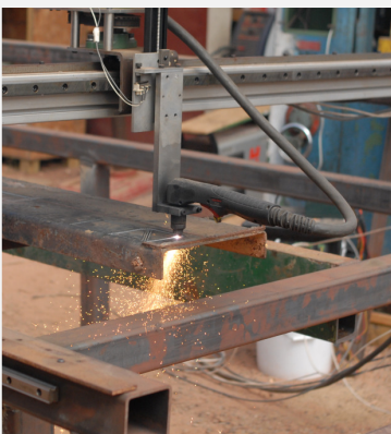
Jason used the partially finished plasma table to make several of the parts needed to finish it. Here's the cutting torch in action.
