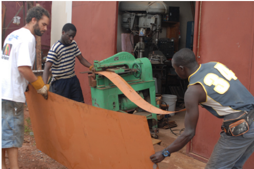
Using the slitter to cut the sheet metal to make the new doors for the discipleship school in Mansoa
