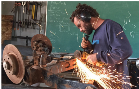
Shortening the axle from a broken-down minivan to use in the donkey cart
