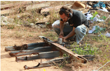
Cutting apart a scrapyard chassis to make the frame for the donkey cart
