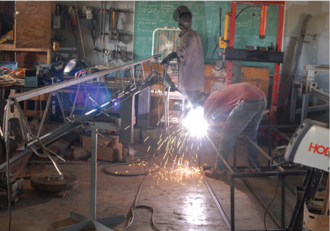
The welding students working on a roof truss and a shelf for the filter factory
