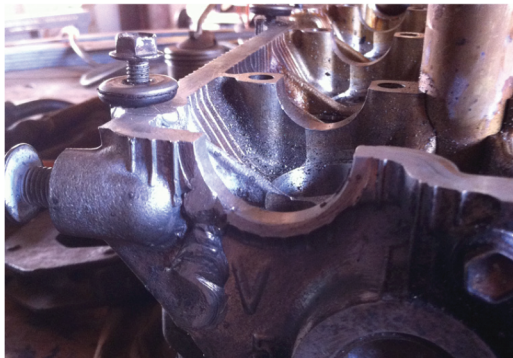
The cast aluminum engine Jason welded back together
