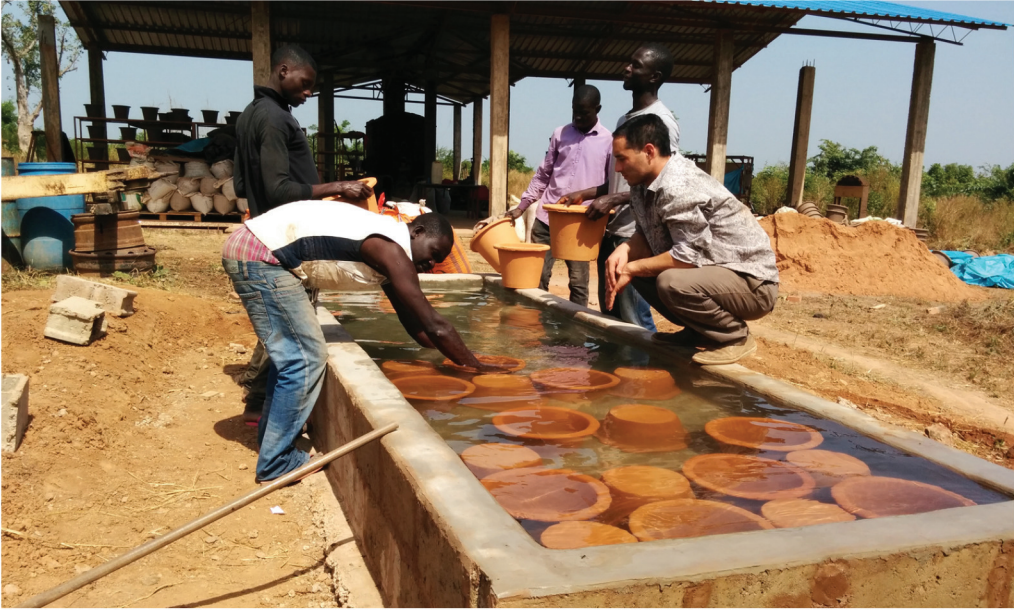
Water filter quality control testing in the dunk tank
