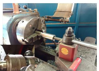
After flipping the new exension around and pressing it on to the shaft, I turned down collars for the bearing journal and the pulley, then cut a keyway.
