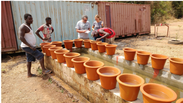
Recording the results of a batch of filter flow tests.
