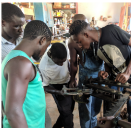
Roughing out the shape of half of the 25mm round tube, 10 thousandths of an inch at a time.
