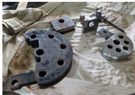
The one from the factory for square tube on the left, and the new one for round tube on the right!
