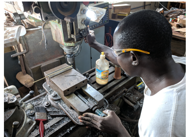
The school's new maintenance guy, Quidam (kee-dahm), getting his first experience on the vertical mill-making brass probes for the pump.
