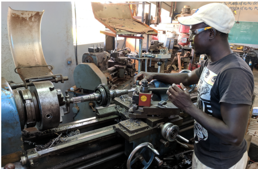
This gearbox shaft had a worn bearing seat which needed to be reduced and a custom bushing mated over it. The end result was perfect!
