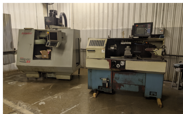
The vertical machining center (left) and CNC lathe (right) safely unloaded at their home for the next year or two.
