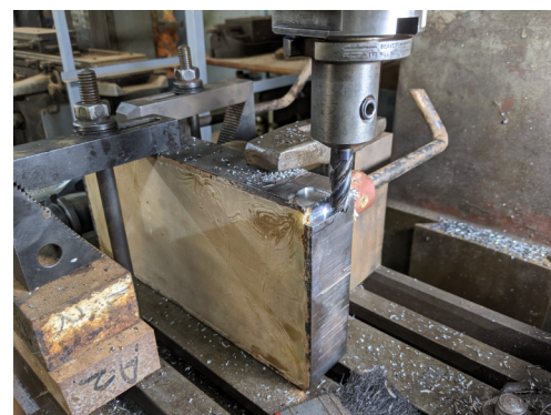
Above I milled a pocket for a replacement for the worn corner in the plate that presses the dirt into a block. Voila!
