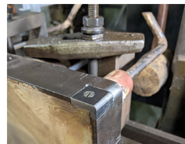
Above I milled a pocket for a replacement for the worn corner in the plate that presses the dirt into a block. Voila!
