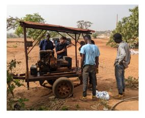
I had my suspicions when this rented generator pulled up. It was supposed to be a 10kva generator but only had a power plug capable of supplying 3kva. Unfortunately, my doubts proved correct the first time we started welding and the tired out old motor bogged down. On to Plan C!
