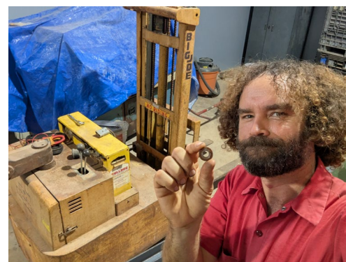
Our aged electric walk-behind forklift stopped working because someone used a steel washer long ago that corroded instead of the proper brass one in an electrical connection! Fortunately, an easy fix after discovering the problem.
