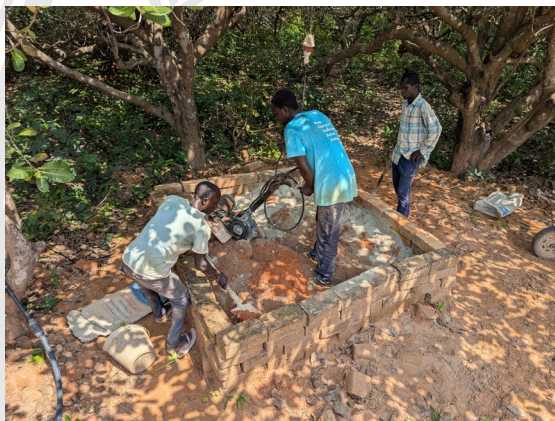
The roto-tiller being converted to use an electric motor has saved a lot of maintenance headaches in such a dusty environment!
