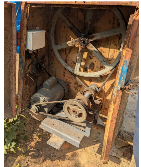
The newly-electrified old cement mixer is lessening our dependence on gas that's sometimes not available, and much quieter to boot!
